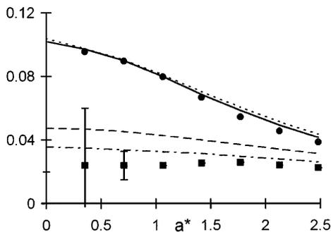
FIG. 1. The kinetic part of  $\psi_1$  ( $\psi_2$ ) as a function of reduced shear rate. The circles (squares) are the simulation results, the full (dashed) line is the result of the moment solution, and the dotted (dot-dashed) line is the result of the kinetic model, Eq. (6).
