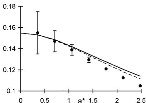
FIG. 2. The kinetic part of the shear viscosity as a function of reduced shear rate. The circles are the simulation results, the full line is the result of the moment solution, and the dashed line is the result of the kinetic model, Eq. (6).
